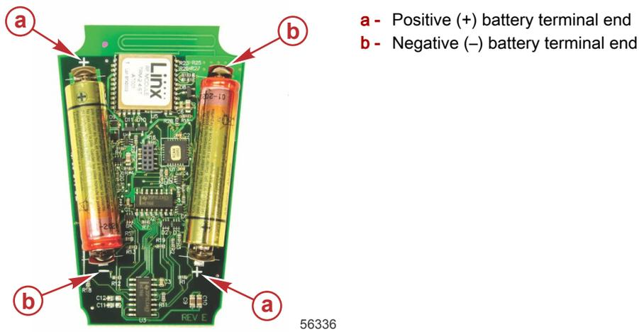
5. Turn the circuit board over and place it gently into the recess in the back cover.
