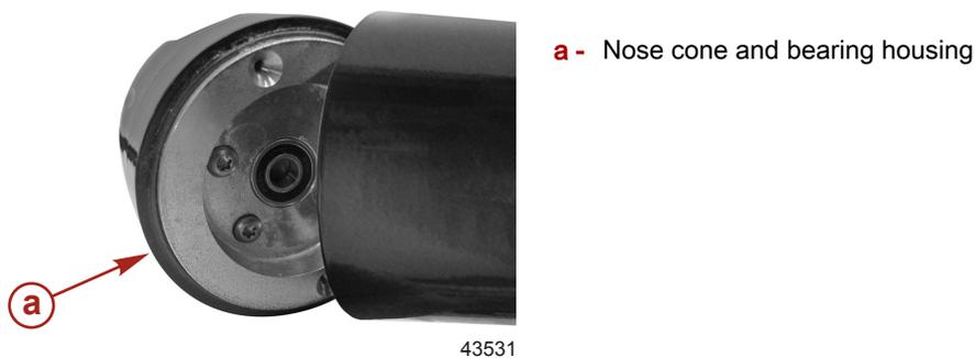
2. Remove the four screws from the bearing housing. Remove the bearing housing from the nose cone. Inspect the nose cone and bearing for damage.
