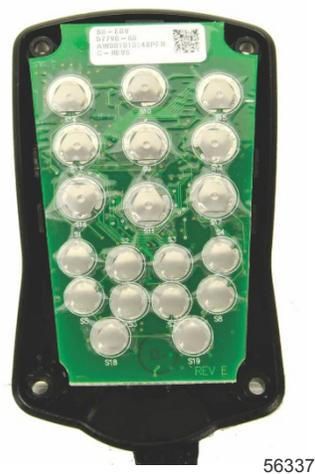
6. Ensure that the rubber seal is seated into the front cover.
