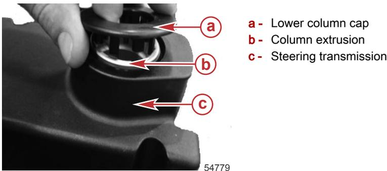
6. Install the column and lower unit from the trolling motor as an assembly. Refer to **Top Housing and Column Assembly**.
