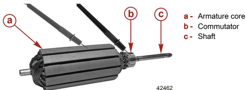
1. With an ohmmeter set on the Rx100 scale, place one probe on the commutator and the other probe on the armature core or the armature shaft.
