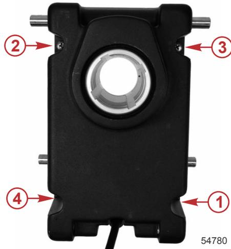
Torque sequence for the steering transmission
