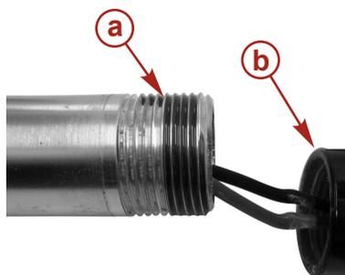
**a** - Loctite 262 on column threads
