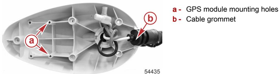
7. Install the top cover onto the trolling motor head and secure it with five #8 x 0.625 in. screws. Ensure that no wires are pinched before tightening the screws to specified torque.
