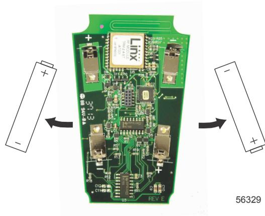
4. Install the new batteries into the battery holders. Ensure that the batteries are installed in the correct orientation.
