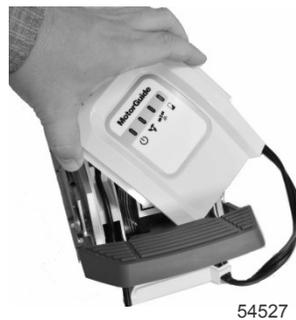
5. Disconnect the GPS module connectors and the status indicator light harness.
