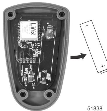
3. Insert the new battery with the positive (+) side facing the positive (+) end of the battery holder.
