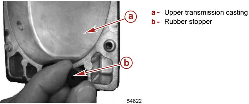
15. Remove the magnet from the slot where the rubber stopper was removed, if replacing the upper transmission casting.
