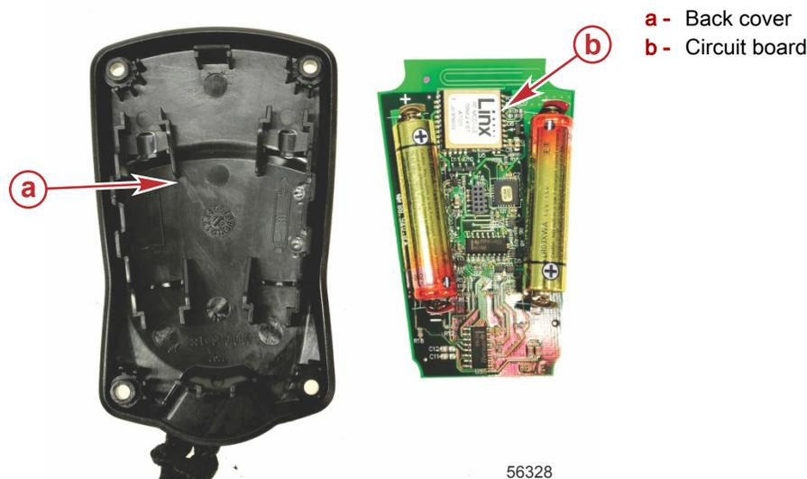
3. Remove the old batteries from the battery holders.
