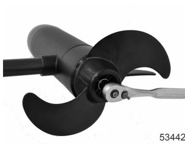
4. Tighten the propeller nut another  $\frac{1}{4}$  turn.
