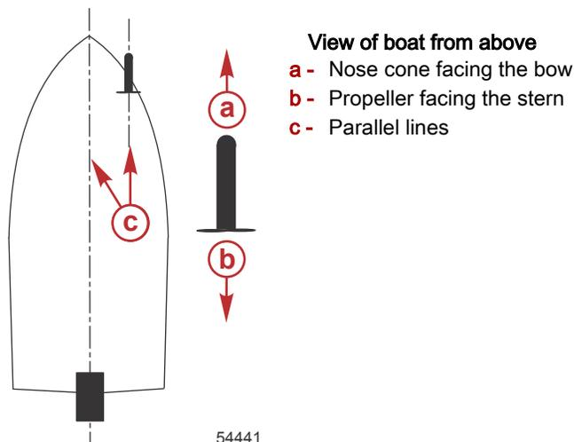
3. Once the lower unit is positioned as close to parallel with the keel as possible, press and hold the **manual mode** button, then press and release the **1, 1**, then **2** buttons in sequence. The trolling motor will emit an audible tune, flash the status indicator light, and then return to manual mode, completing the mounting angle calibration.
