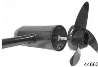
3. Install the washer (or anode, for saltwater models) onto the propeller shaft then install the propeller nut. Tighten the propeller nut securely.
