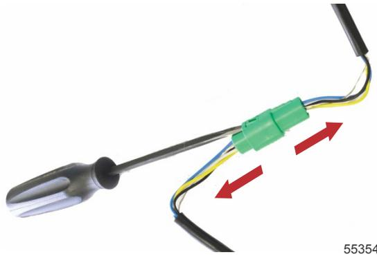
8. Remove the cable grommet from the trolling motor head.
