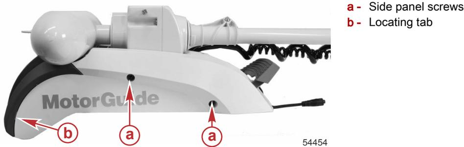
4. Remove the five screws securing the top cover to the trolling motor head.
