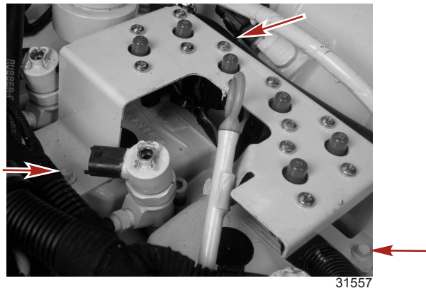
Circuit breaker panel screws
