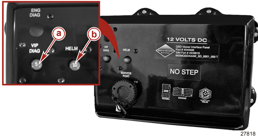
Vessel Integration Panel (VIP) circuit breakers
