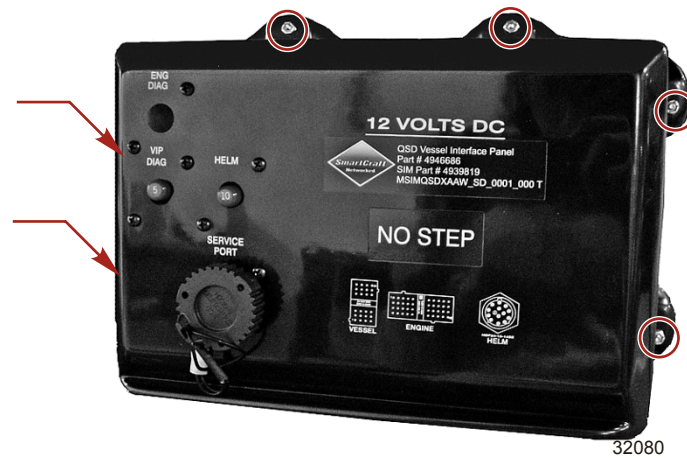
VOP mounting screws (6 total, 2 not visible)
