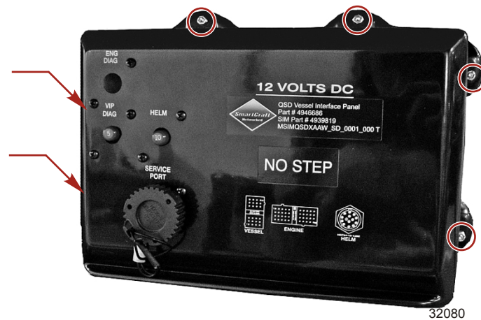
VOP mounting screws (6 total, 2 not visible)
