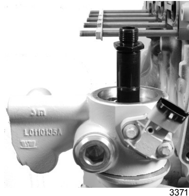
Loose oil feed pipe and cooler housing
