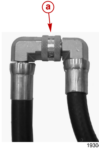
a - Hydraulic lines quick-connect fittings
