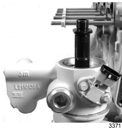
Loose oil feed pipe and cooler housing
