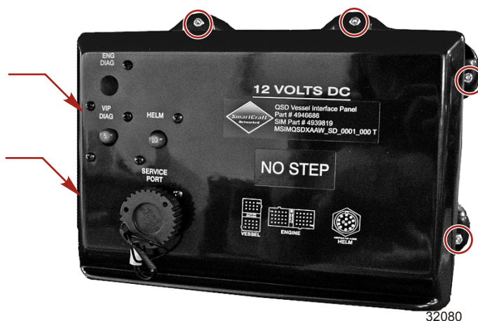
VOP mounting screws (6 total, 2 not visible)
