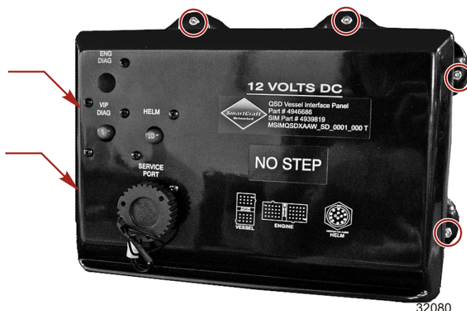
VOP mounting screws (6 total, 2 not visible)
