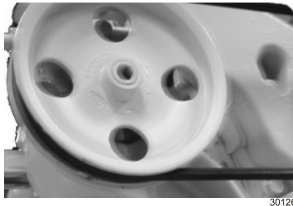
Pulley installed flush with shaft end
