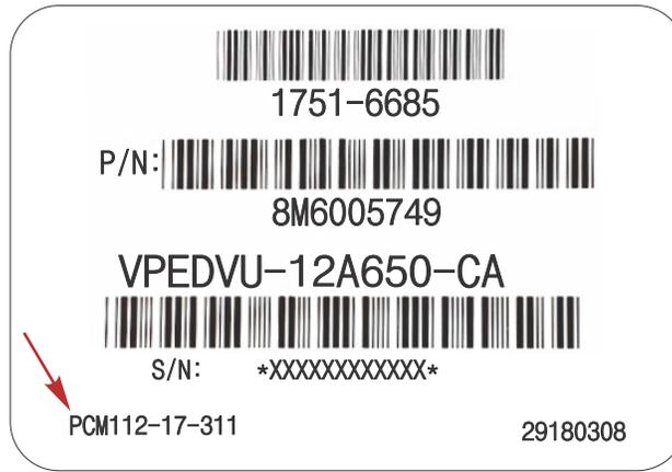
PCM label: The number in the lower left identifies the controller: PCM 112. The next two digits are the year it was introduced. The last three numbers are an internal cross-reference number.
