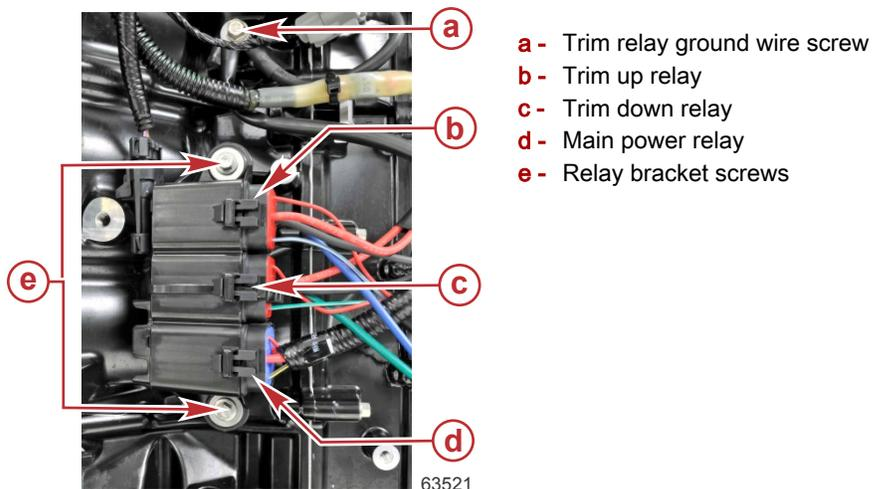
The trim motor relay system, used on permanent magnet trim systems, connects each of the two wires from the trim motor to either ground or positive to allow the motor to run in both directions.
