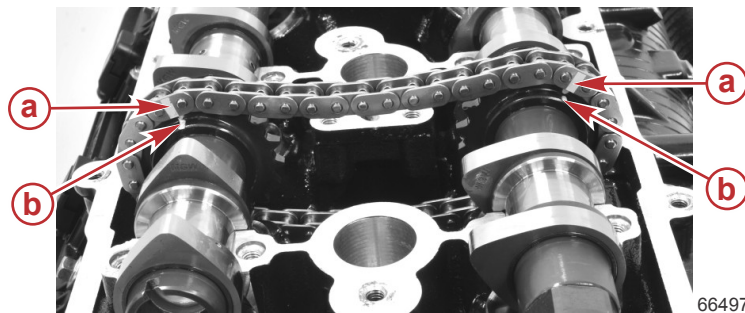
Port camshafts in TDC position (V8 shown—V6 similar)
