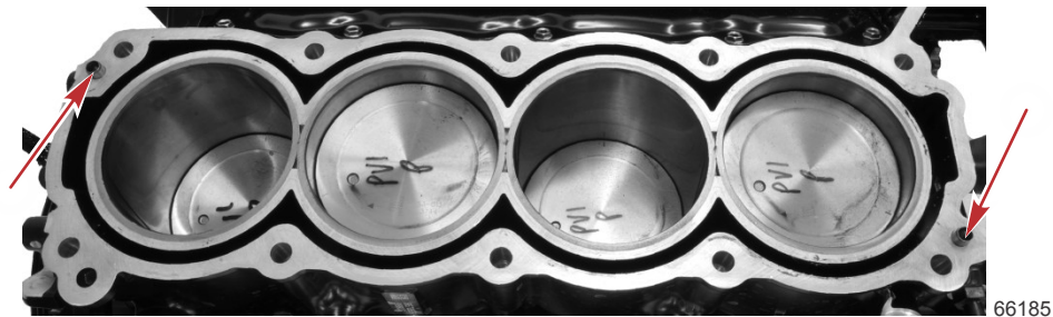
Dowel pins (two per bank) (V8 shown—V6 similar)
